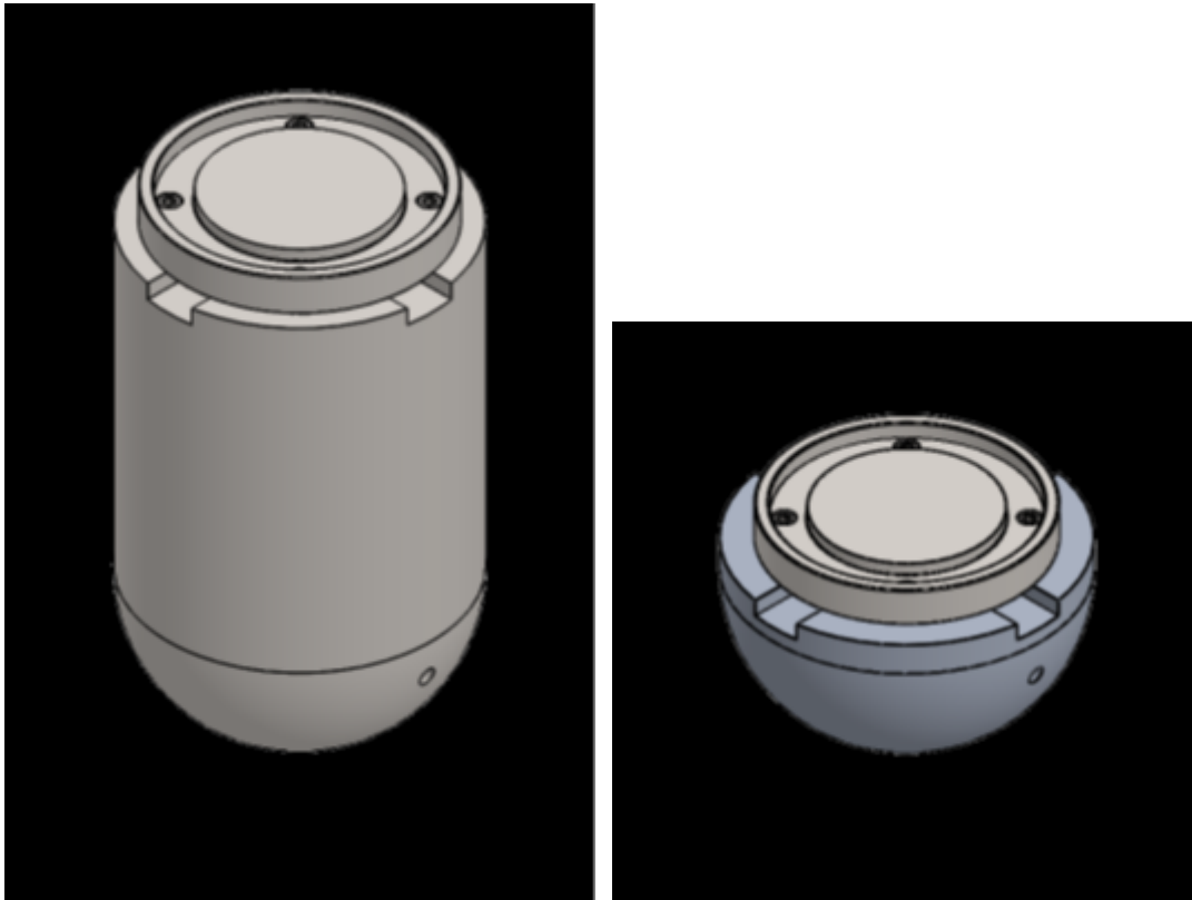
Fig.2 Depiction of the impactors used for testing, EN 12572-2:2017 [2], and NF P90-311:2009 [3] on the left, and AS2319.1-2009 [5] and EN 1177:2018 [6] on the right.
